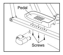
forward or backward to the desired position, and reattach them with the screws. Make sure that both pedals are in the same position.
